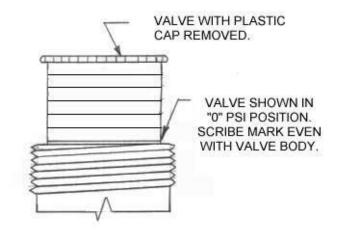
valve setting and operation. The valve may need to be cleared of dirt or chips if adjustment is not possible. With the compressor running, turn the valve adjustment knob clockwise about 3 turns momentarily then back to the proper setting. Do not leave the valve in open position (allowing high backpressure) as this may cause the compressor to overload.
