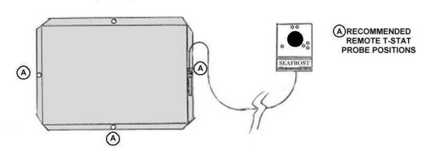
**WIRING:** Connect the thermostat wires at the compressor module to terminals T & C using female 1/4" crimp connectors. There is no polarity requirement.
