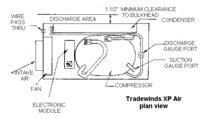
An un-ducted unit in a poorly ventilated small space will heat the air, thereby lowering the capacity of the unit and possibly causing damage by over-heating the compressor.
