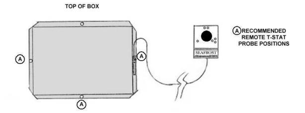
The SEA FROST BD thermostat is variable. Turning the knob fully counterclockwise turns the unit "OFF". The full clockwise setting is the coldest. The thermostat may be adjusted to obtain any temperature desired in the cabinet. The thermostat may be calibrated should the warmest setting be too cold. To calibrate the thermostat remove the mounting screws and tip the panel forward. Remove the electrical tape (if necessary) the adjustment screw about an inch into the case.
