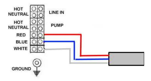
With other thermostats connect the blue and red wires only to a make and break switch. This is normally closed. Do not apply power to the red, white or blue terminals. Do not connect the white terminal.
