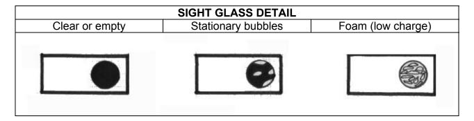
A clear sight glass, when the compressor is operating, signifies a sufficiently charged system. To determine the meaning of "clear", notice the appearance of the RFD sight glass when the system is at rest with the compressor off. This is a "clear" glass.
