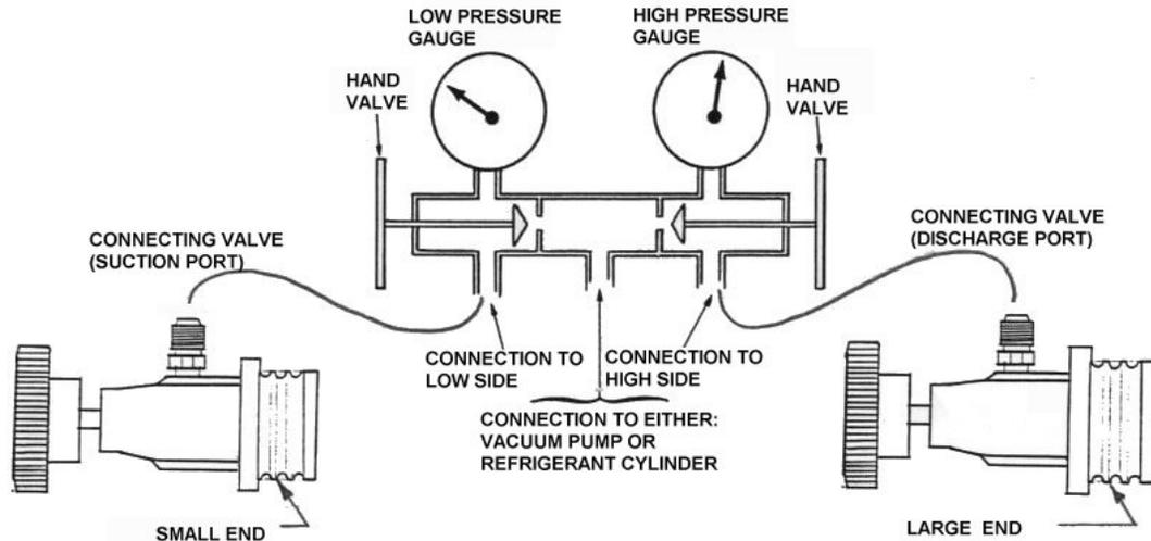
Gauges are used in the evacuation and charging. They will provide information on the operation of the system.
