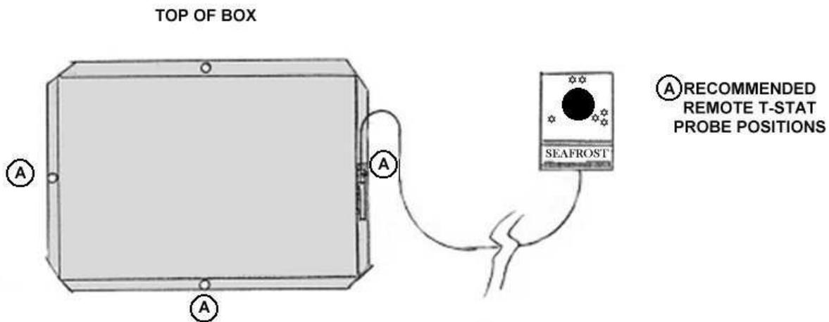
The SEA FROST BD thermostat is variable. Turning the knob fully counterclockwise turns the unit "OFF". The fully clockwise setting is the coldest. The thermostat may be adjusted to obtain any temperature desired in the cabinet. The thermostat may be calibrated should the warmest setting be too cold. To calibrate the thermostat remove the mounting screws and tip the panel forward. Remove the electrical tape (if necessary) to expose a black adjustment screw about an inch into the case.
